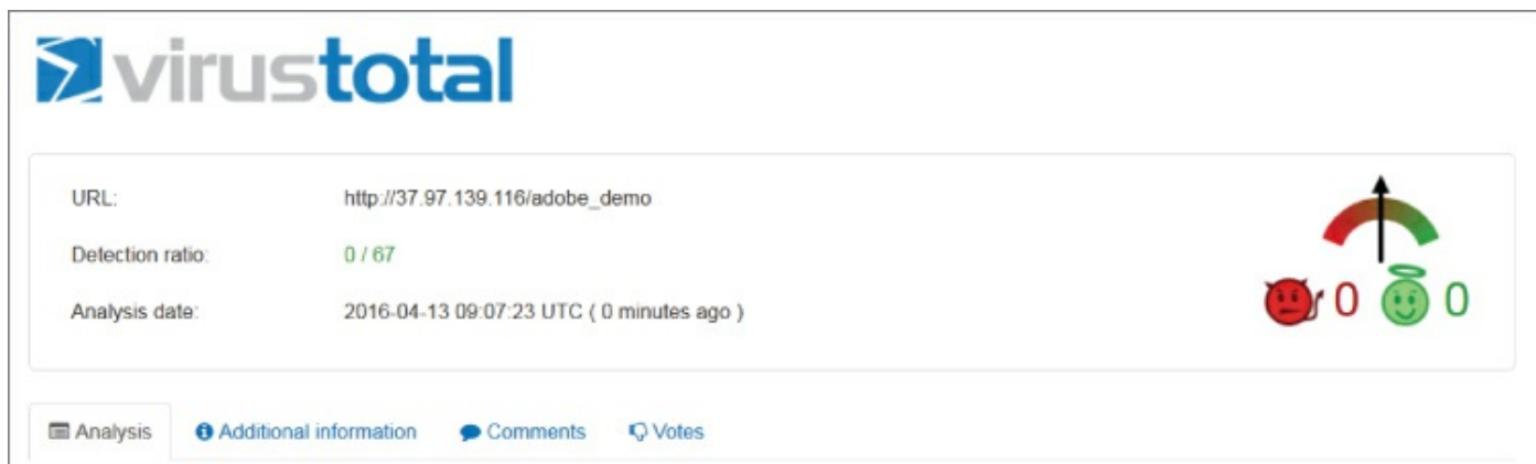
Figure 4.7: Metasploit does an excellent job at obfuscating the CVE-2015-5012 attack.
