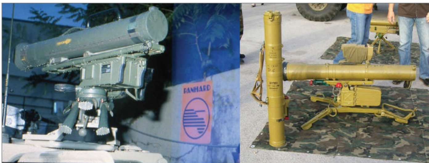
Figure 5.2: The Soviet AT-4 (right) was a copy of the French MILAN system (Left).
