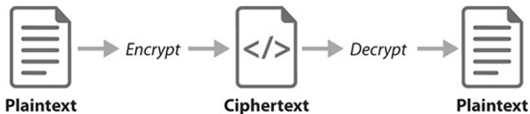
Figure 4-2 Encryption and decryption
