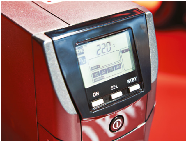
FIGURE 8.6 Uninterruptible power supply (UPS)
