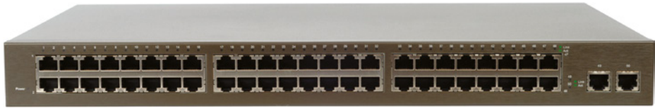
FIGURE 16.4 A 48-port network switch
