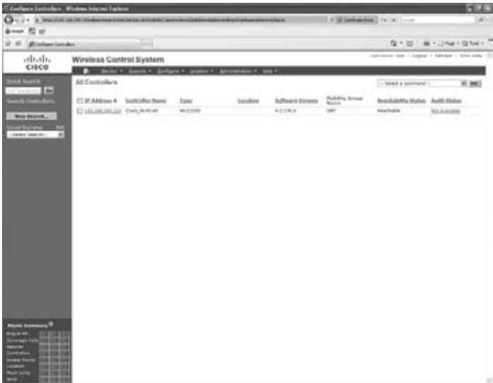
FIGURE 20.19 All Controllers with a WLC
