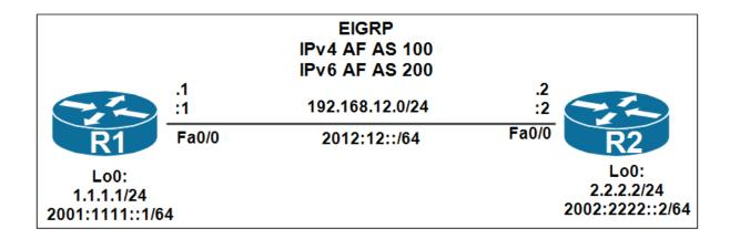
R1 and R2 are using EIGRP Named Mode for both IPv4 and IPv6 Address Families using the router eigrp CCIE command.
