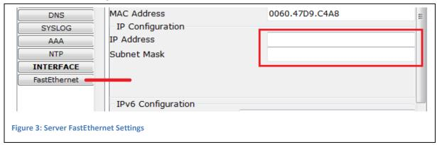
As seen in Figure 3, in this window, you can configure the settings for the Ethernet card for Server 1. Use the Addressing table on Page 1 to fill in the IP address and subnet mask for Server1.
