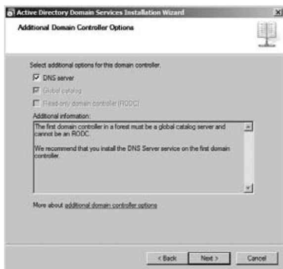
Figure 11.8: Installing AD with DNS
