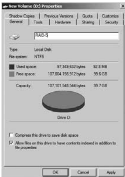
Figure 9.12: RAID 5 drive size
