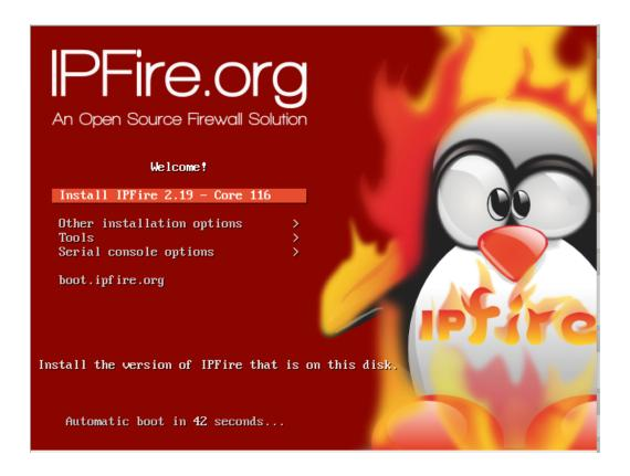
IPFire is completely free of charge, and it only takes a few minutes to set up. You install it on a machine with at least two network interface adapters and configure it to match your network configuration. It's a proxy-type of a firewall, which means that in addition to doing normal firewall-type packet inspection, it also includes caching, content-filtering, and NAT capabilities. You can set up IPFire in a number of different configurations:
