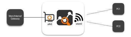
To properly operate in 1+1 mode, eth0 must be added to a linux bridge before firing up ntopng. This is accomplished by editing file /etc/network/interfaces as follows:
