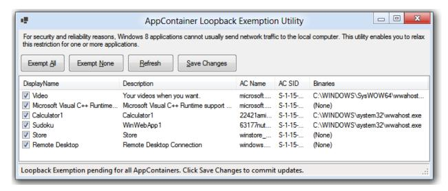
App Container is the security sandbox within Windows 8 that hosts apps. It offers fine-grained security permissions and blocs write and read access to most of the system when using an app. By default, an app can only access its AppData folder and cannot directly access anything else in the system unless the user grants it access.
