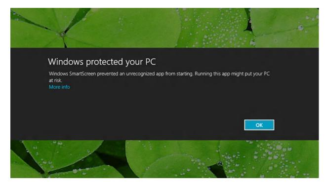
SmartScreen is a phishing and malware filter included as part of the Windows 8 operating system. It is designed to help protect users from attacks associated with downloads that infect a system. In Windows 8 it filters at the desktop level, checking the reputation by default on any file or application downloaded from the internet.
