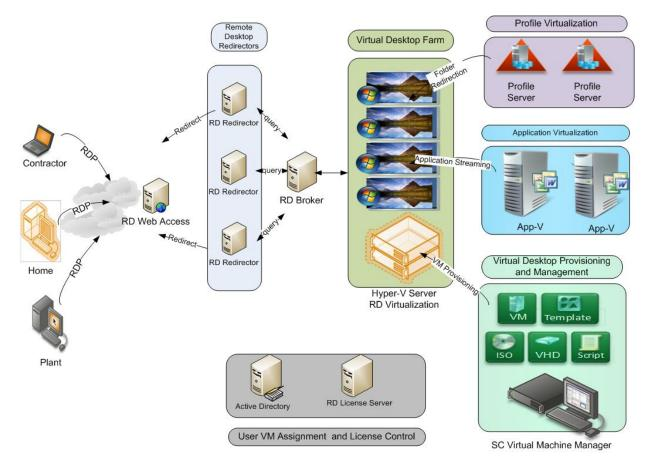
Microsoft included a variety of Virtual Desktop Infrastructure (VDI) enhancements in Remote FX and Windows Server 2012 with this round of upgrades and new releases. These enhancements improve the desktop experience of users by allowing 3D graphics, USB peripherals, and touch enabled devices across any type of network.
