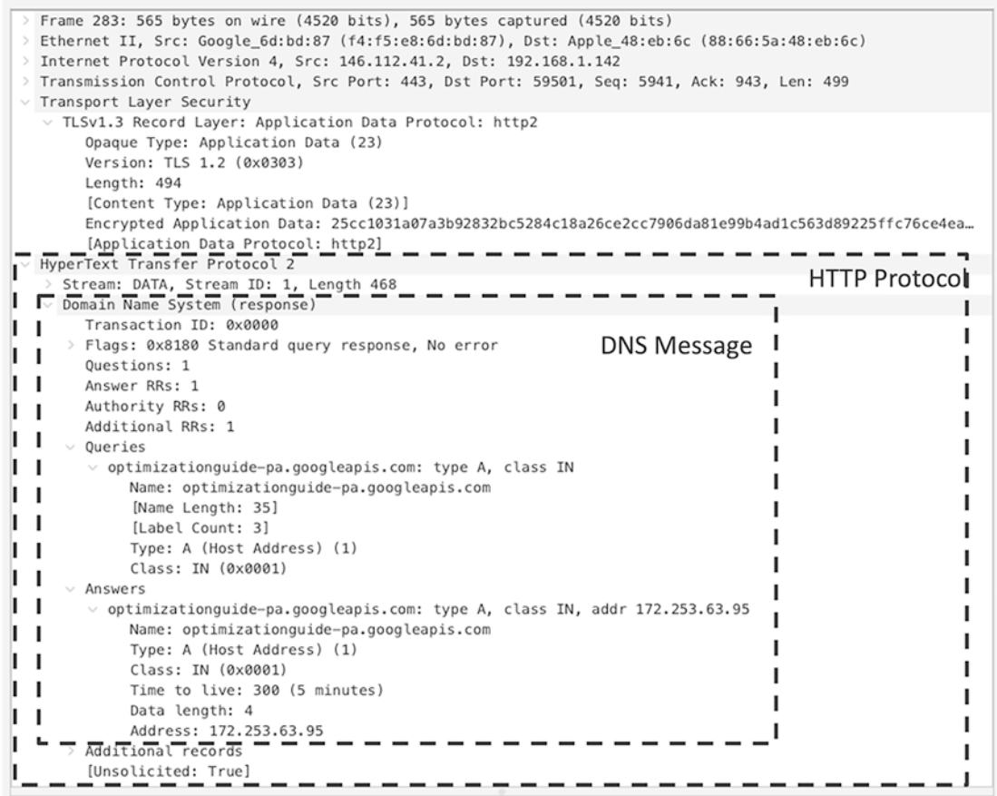
Figure 3-31. Wireshark capture for Secure DNS
